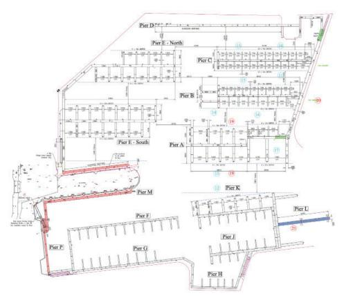
This final phase marked the end of an extend and refurbishment project that began five years ago. Built with Walcon's durable System 21 pontoons fitted with composite decking specified by the client, it will be extremely hard-wearing for many years to come. Other high quality features include a striking bow-string bridge that complements
