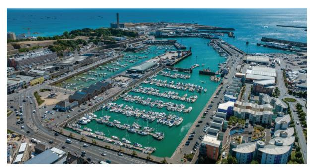
The overall scope required the removal and replacement of the entire on-the-water infrastructure. This included all the pontoons as well as the existing guide piles that had also reached the end of their serviceable lives. The two existing access bridges were refurbished and reinstated by Geomarine. In all, around £3.5m was invested in the project to enhance the facilities, and the project was completed on time in May.
