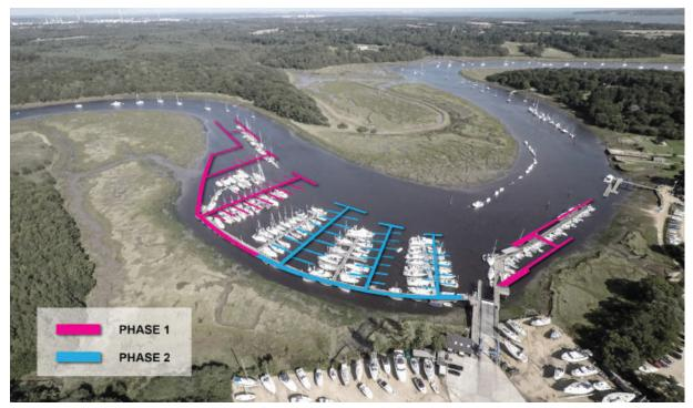
The following year stage two began with the removal and subsequent reinsertion of the back walkway so as to manoeuvre the phase one pontoons in position. This was then followed by the removal of piers A, B and C, and the continuation of the process of refurbishing the pontoons to be re-used, driving the new piles, and the reassembly of the piers with their extensions.
