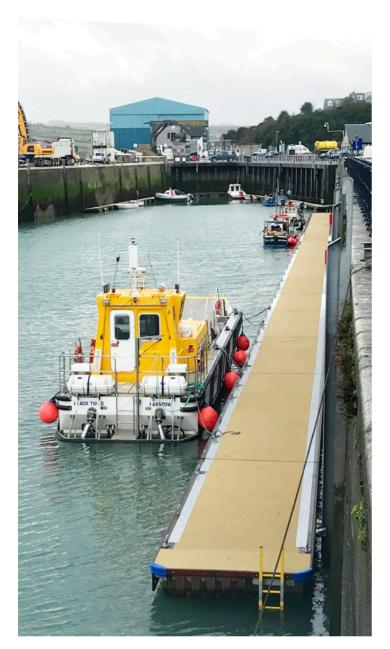
Additional features for these workboatgrade pontoons include an all-round timber skirt to protect the floats and three-tonne mooring cleats.
