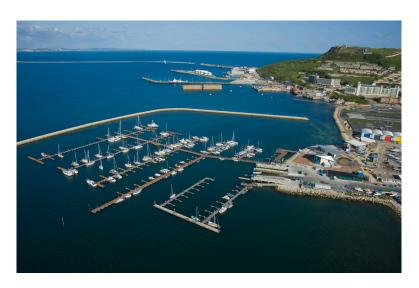
As an additional detail the outermost pontoons, intended to provide berthing for larger yachts, have been specially modified to give a freeboard of 650mm versus the conventional 500mm.
